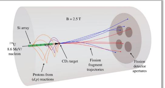
Example particle trajectories in HELIOS@ANL for reactions populating the ground state in <sup>239</sup>U (orange) and states close to the fission barrier (purple) Example fission fragment trajectories for fragments with A=138 (red) and A=100 (blue), for a range of emission angles.
