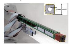
For **y-rays**: Apollo scintillator array, 5 LaBr + 15 Csl
