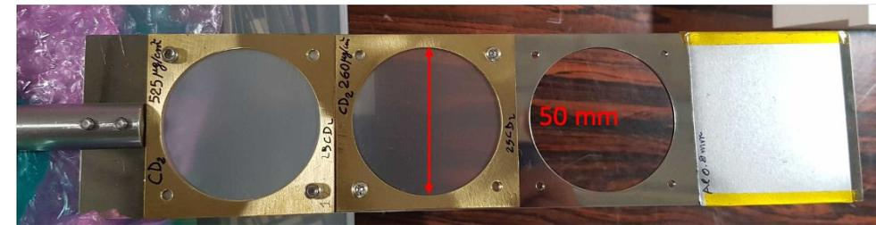
Target holder with the CD<sub>2</sub> secondary target.
