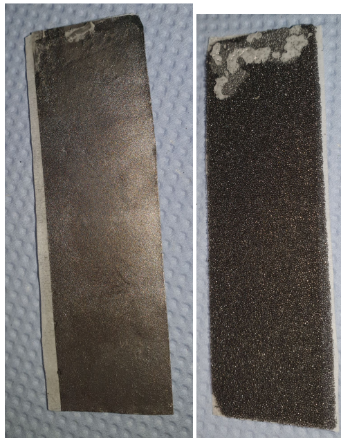
FIGURE 3.16 – Left: The front of the PGS/RVC sample. On the left side of the sample the ply sheet is visible. Right: The bottom of the PGS/RVC sample. Visible is the RVC and the glue (top) in the clamping area used to reinforce the foam structure.
