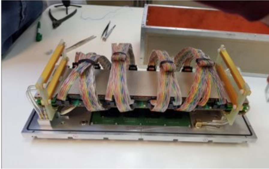
Figure 5.3: A photo of the direct flow prototype MSMGRPC of 56 mm strip length after assembling.
