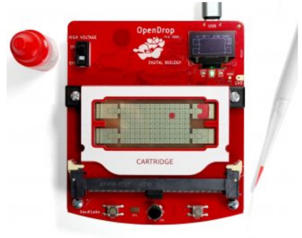
OpenDrop V4 – Digital Microfluidics Platform
