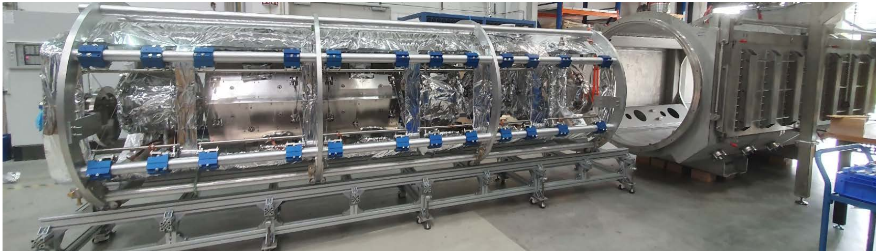
Acceleration string mounted inside transport frame
