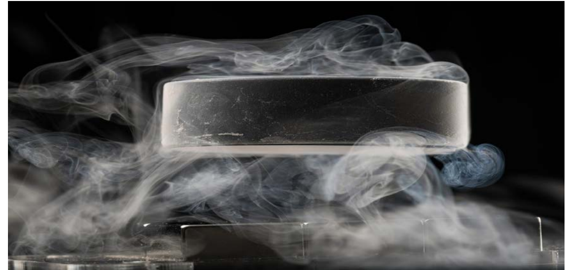
Magnets are seen suspended above a track in a superconductivity demonstration kit in a lab at the University of Rochester. The primary researcher, Ranga Dias, is pursuing his goal to create novel quantum materials such as superconductors with a critical temperature at or near room temperature.
