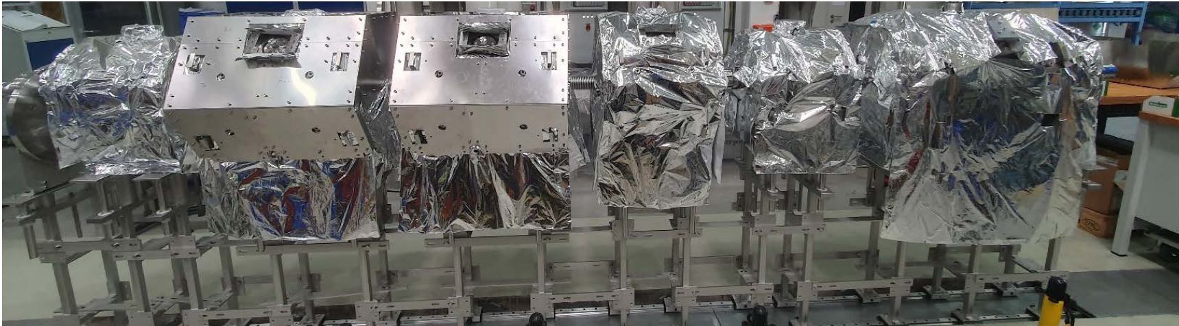
Acceleration string mounted on individual trolleys
