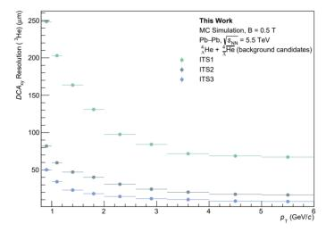
Fig. 16: Transverse-plane impact-parameter resolution for primary (background) <sup>3</sup>He particles from  $^{4}_{\Lambda}$ He decays for ITS2 (green circles) and ITS3 (blue squares) as a function of  $p_{T}$ .
