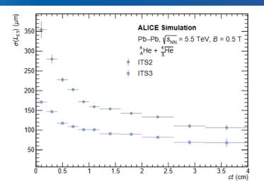
Fig. 17: Resolution on the  ${}^{4}_{\Lambda}$ He-candidate decay length in the *xy* plane for ITS2 (green circles) and ITS3 (blue squares) as a function of  $p_{T}$ .
