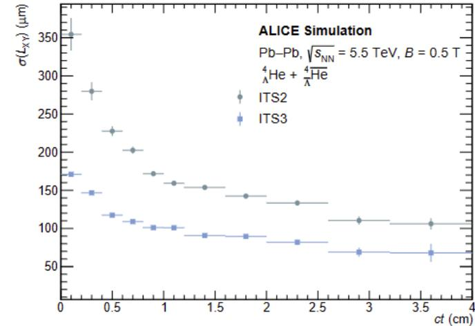
Fig. 17: Resolution on the  ${}^4\text{He}$ -candidate decay length in the  $xy$  plane for ITS2 (green circles) and ITS3 (blue squares) as a function of  $p_T$ .
