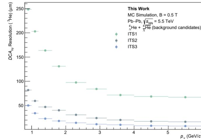
Fig. 16: Transverse-plane impact-parameter resolution for primary (background)  ${}^3\text{He}$  particles from  ${}^4\text{He}$  decays for ITS2 (green circles) and ITS3 (blue squares) as a function of  $p_T$ .
