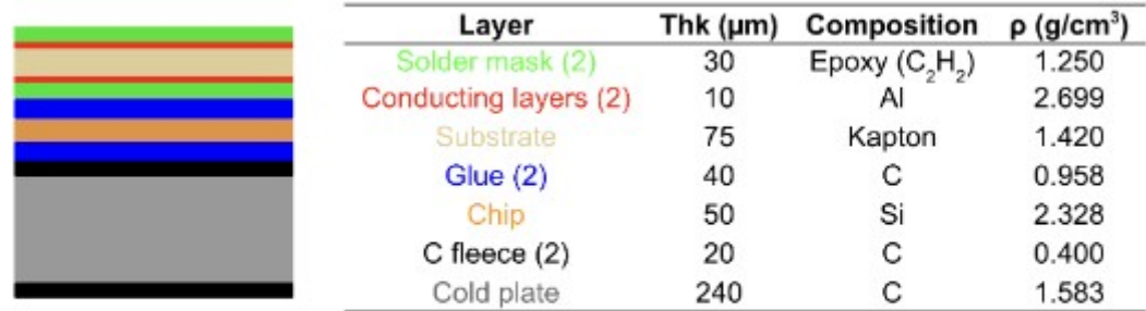
Figure 4.5: The stack of ALPIDE layers, as defined in the simulations
