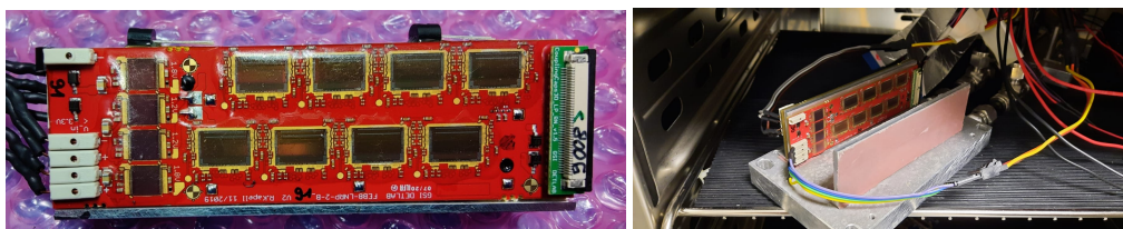
Figure 4.23: A FEB glued to the T-shelf, with 3 DS18B20 temperature sensors installed on the T-shelf (left) and two FEBs mounted on a T-shelf with thermal pads inside a climatic chamber (right).
