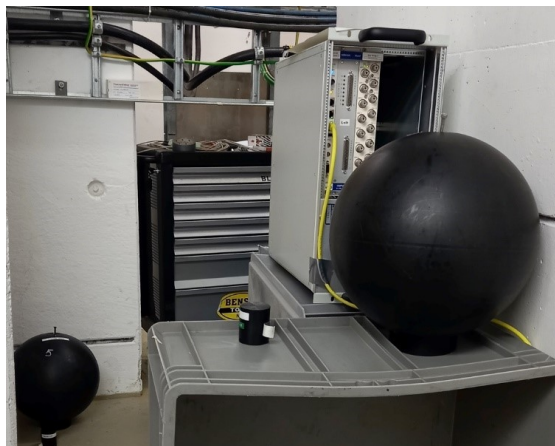
Figure 4.3: Crate irradiation setup at the mCBM experiment. The photo depicts two TLD dosimeters in the background, and two TLD dosimeters and the crate in the foreground.
