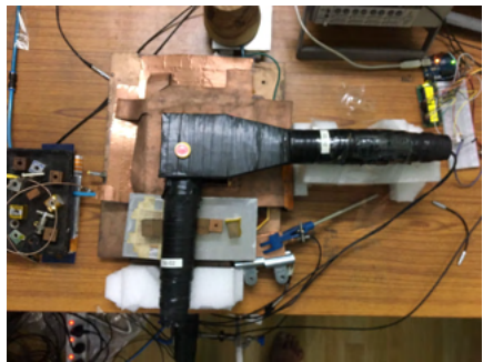
Figure 4.14: Left: Detector arrangement for the time resolution measurement of SM triple GEM chamber. Right: Schematic of the electronics setup for the time resolution measurement of SM triple GEM chamber. The ^{137}\text{Cs} source is placed on top of scintillator SC3.
