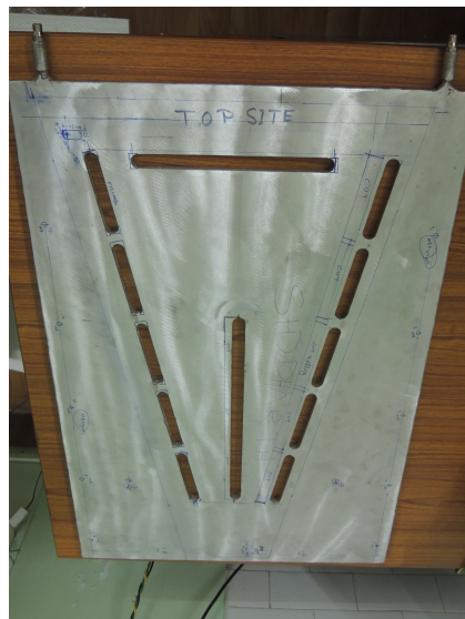
Figure 3.7: Sample cooling plate after fabrication using technique II.
