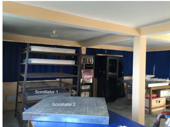
Figure 3.15: Horizontal stack of three scintillator detectors to measure cosmic ray shower.
