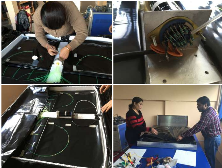
Figure 3.9: Construction of PSD modules: (Top left) WLS fiber insertion, (Top right) Voltage divider network, (Bottom left) HV cable connected in proper position, (Bottom right) Closing the box.
