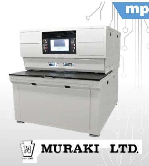
Multi-Point Compensating X-Ray 2-Spindle Drilling Machine
