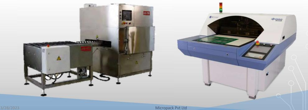
100% BBT by Flying Probe testers / grid tester – Max panel size upto 810x510mm Pre-despatch Inspection – Full fledged microsection / Visual inspection facility Impedance measurement – Using Polar 800 Si
