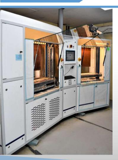
Non-conductive Via Filling – with Taiyo THP 100 paste
