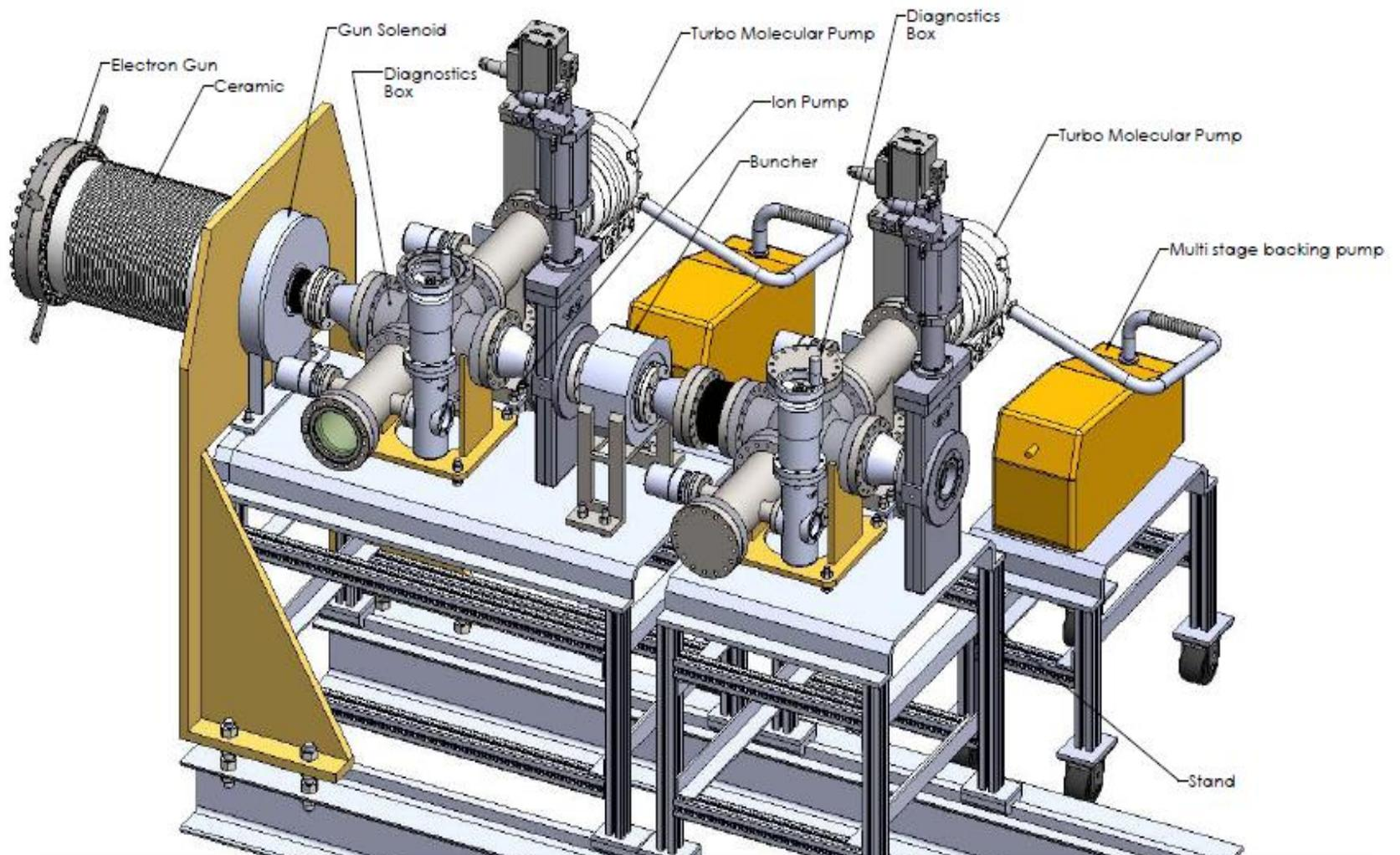
**100 keV electron gun and LEBT line for VECC's 10 MeV Injector**
