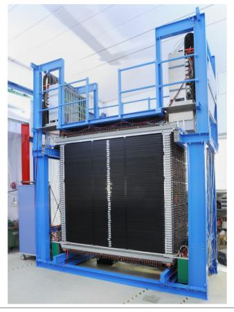
Double plane:  $1^{st}$  plane  $\rightarrow 50$  horizontaly oriented bars  $2^{nd}$  plane  $\rightarrow 50$  vertically oriented bars
