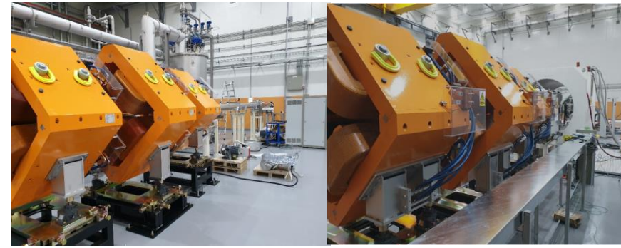
Beamline (Left: IF side, Right: LAMPS side)
