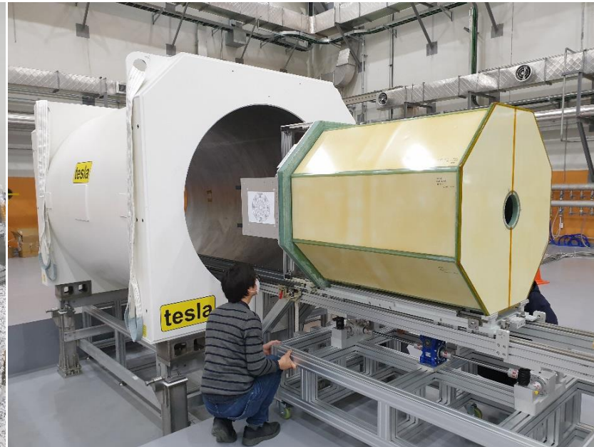
Installation of TPC inside the magnet
