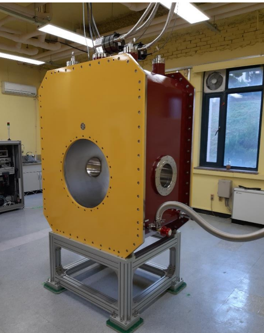
Low-energy detectors (Left) SC magnet with B_{max} = 1.5 \text{ T} (Above) AT-TPC (prototype)
