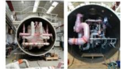
Cold Box (CB) (Left warm side, right – cold side)
