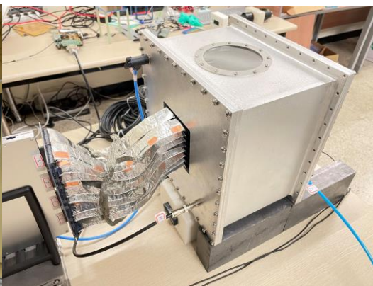
Low-energy detectors (Left) SC magnet with B_{max} = 1.5 \text{ T} (Above) AT-TPC (prototype)
