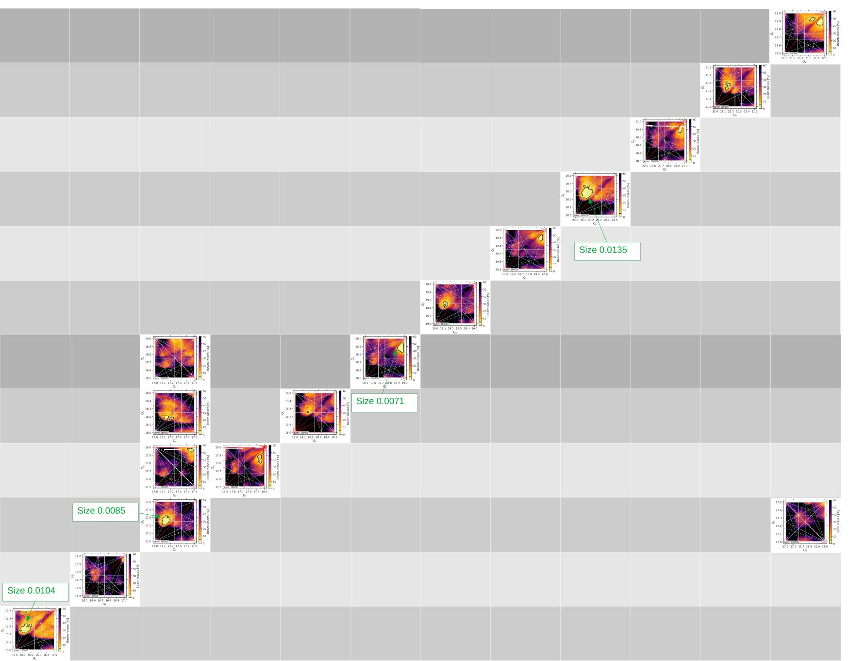
**Tune diagrams** for U28+ at nominal fast extraction parameters (0.3 max. SC tune shift)
