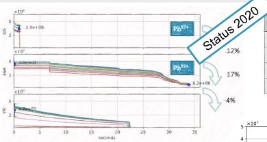
Loss per Resulting beam step in % intensity in % One out of two bunches 50 % 50 % HEST GHTYDC1-DC2 45 % 27.5 % Injection/bunching 20 % 22 % Unidentified Loss Factors 82 % 4 %
