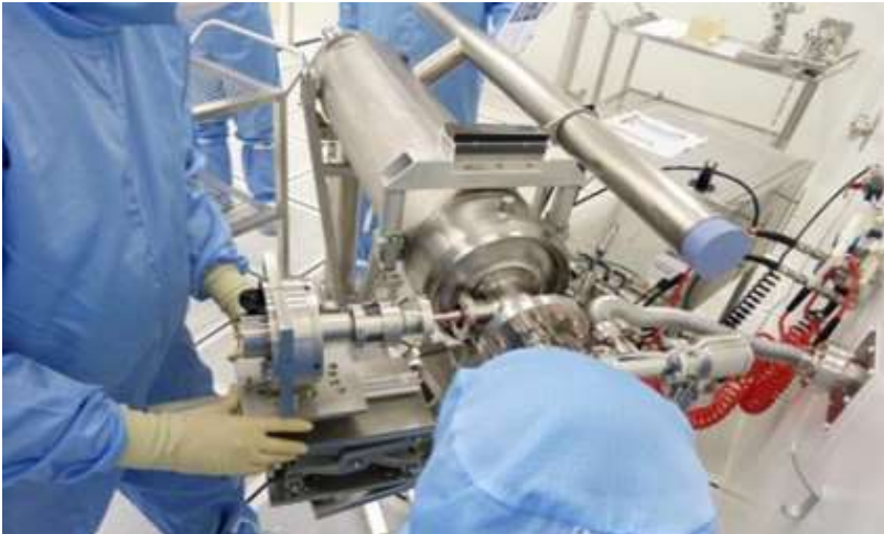
Assembly of the XFEL cryomodules
