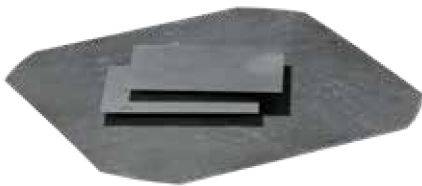
Test plate made of silicon nitride
