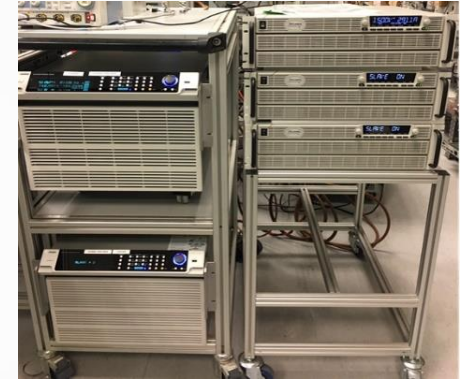
Project with TDK Lambda for 30 devices 500A/50V controlled by REGUL8OR
