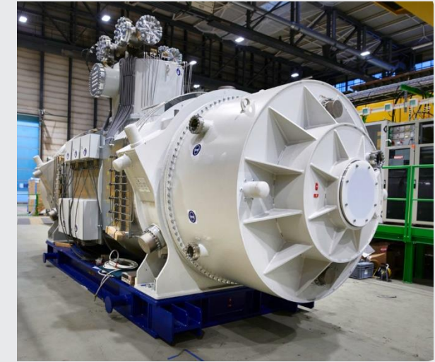
upto 9 magnets in one cryostat
