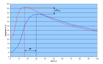
Comparison of the heat of hydration of a cooled (blue) and an uncooled concrete (red) Gases for Life
