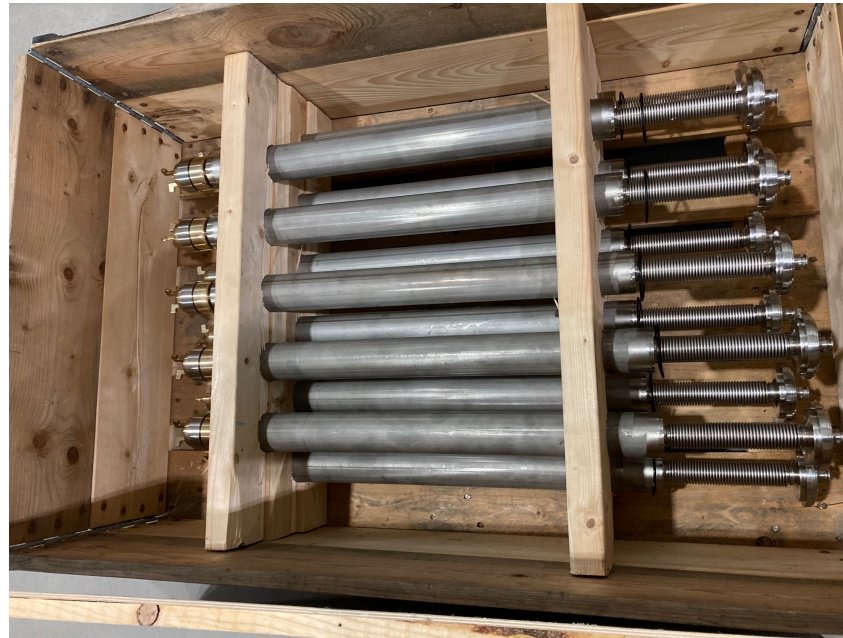
First batch of dismantled valve stems
