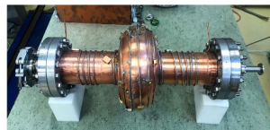
Radiofrequency 1.3 GHz prototype cavity with soldered cooling capillaries
