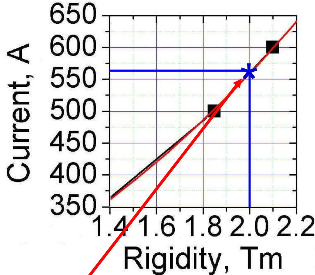
Simulated calibration curve for dipole magnet with error < 1%
