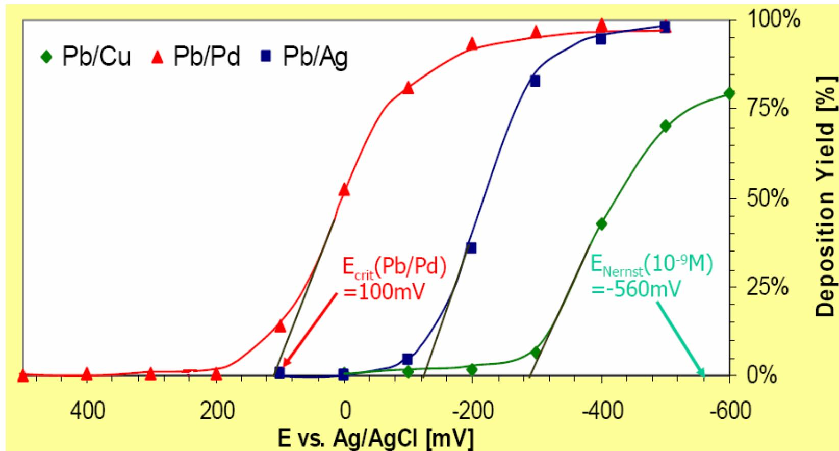
Deposition of  $^{212}\text{Pb}$  on Pd, Ag and Cu from 0.1 M  $\text{HClO}_4$
