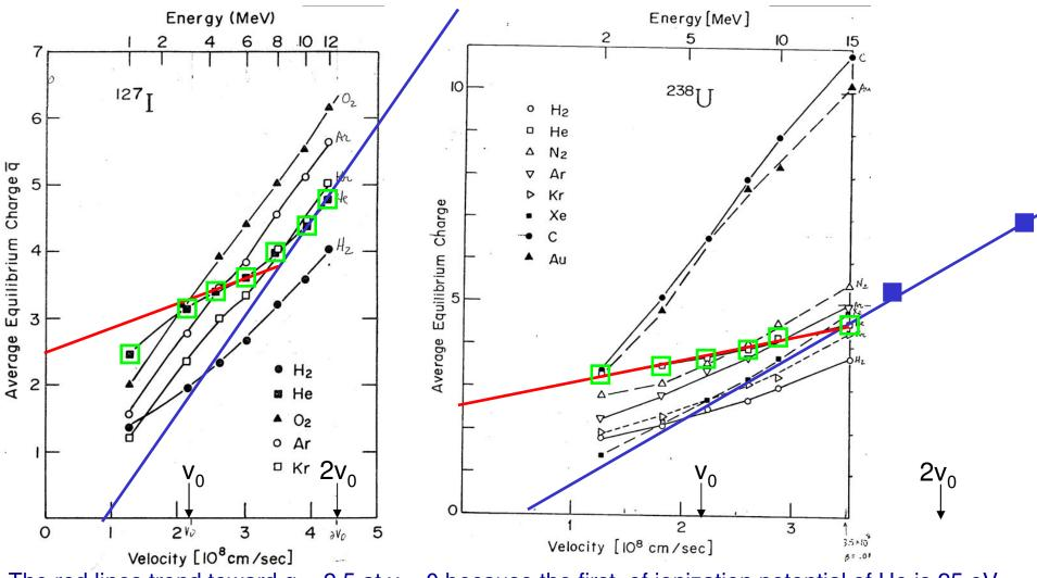
The red lines trend toward q = 2.5 at v = 0 because the first of ionization potential of He is 25 eV. This is usually between the second and third ionization potentials of heavy elements.
