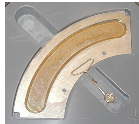
Thin ^{249}\text{Cf} target used as reference
