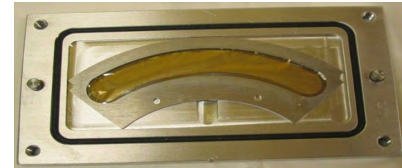
^{249}\text{Bk} target used as reference
