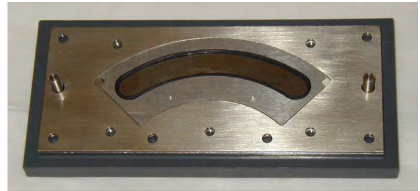
Target-segment on cathode-plate (Ti) with distance frame (Ti)
