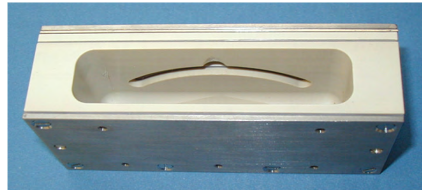
Molecular Plating cell with Ti-foil as cathode and Pd-foil as anode
