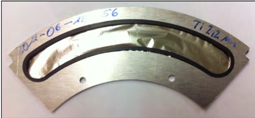
Target-segment with 2.3 \mu\text{m} Ti-backing-foil and Viton-O-ring
