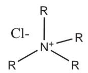
$R = C_8 H_{17}$  and  $C_{10} H_{21}$
