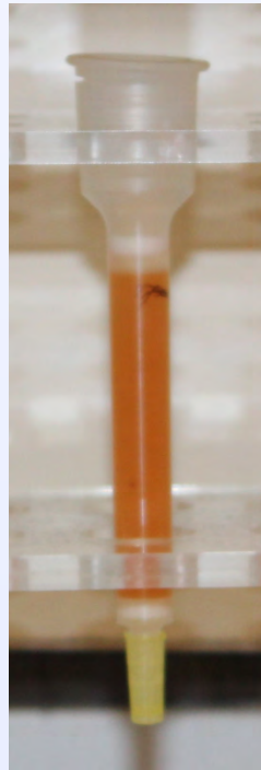
AG 50w x 8 generator
