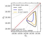
**Figure:** low-loss area with warm quadrupoles
