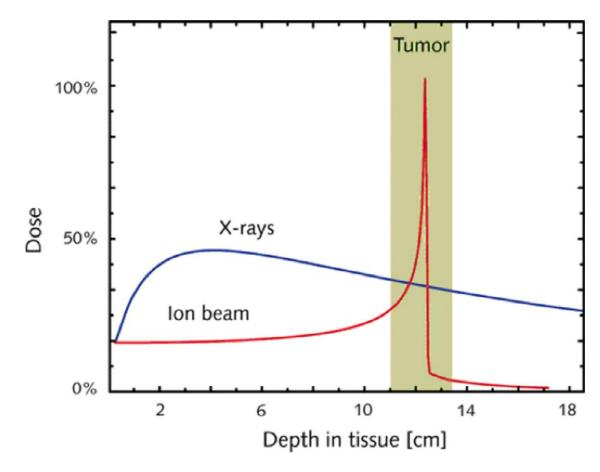
Depth dose distribution of high-energy photons vs charged particles.
