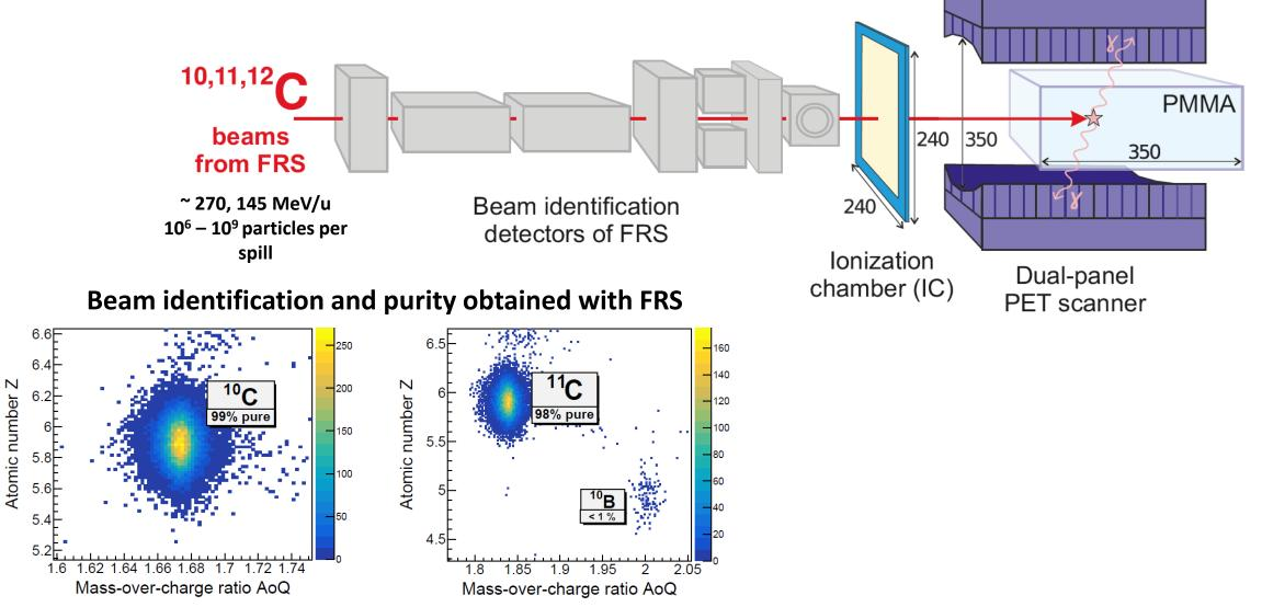
Idea of the measurement: in-beam PET imaging using positron-emitting isotopes of carbon.
