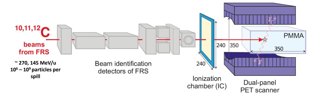
Idea of the measurement: in-beam PET imaging using positron-emitting isotopes of carbon.
