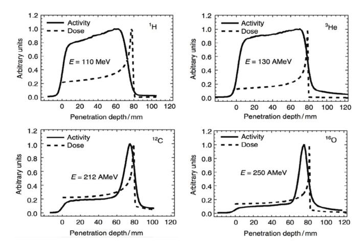
Measured activity and dose profiles in PMMA for protons, <sup>3</sup>He, <sup>12</sup>C and <sup>16</sup>O Figure from [Fiedler F. et.al., Ion Beam Therapy 527, (2012)]
