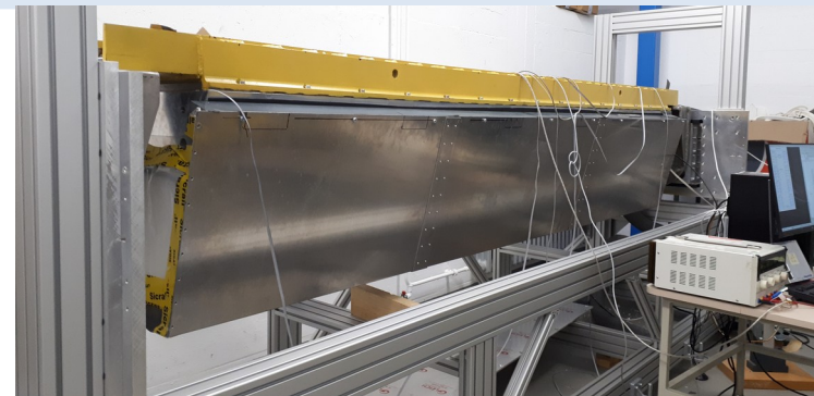
Relative Humidity in the Slice measured with PANDA THMP
