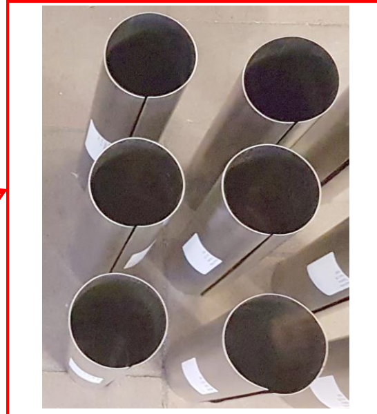
Picture 4: Vacuum pipes before welding Wall thickness 0,85 mm Inner diameter 77,3 mm
