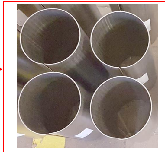
Picture 5: Vacuum pipes before welding Wall thickness 2 mm Inner diameter 140 mm
