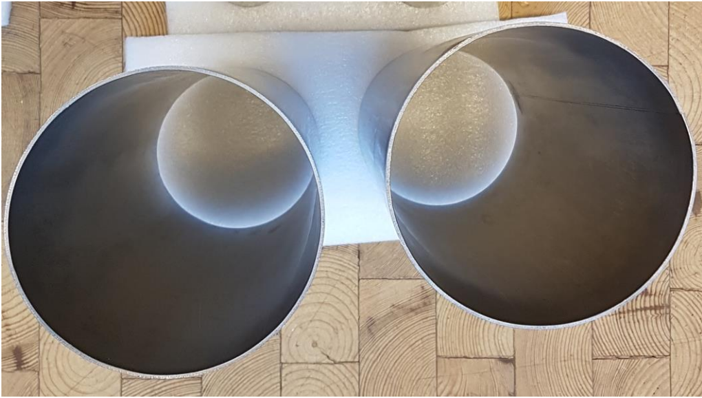
Picture 6: Vacuum pipes welded and rerolled Wall thickness 2 mm Inner diameter 140 mm
