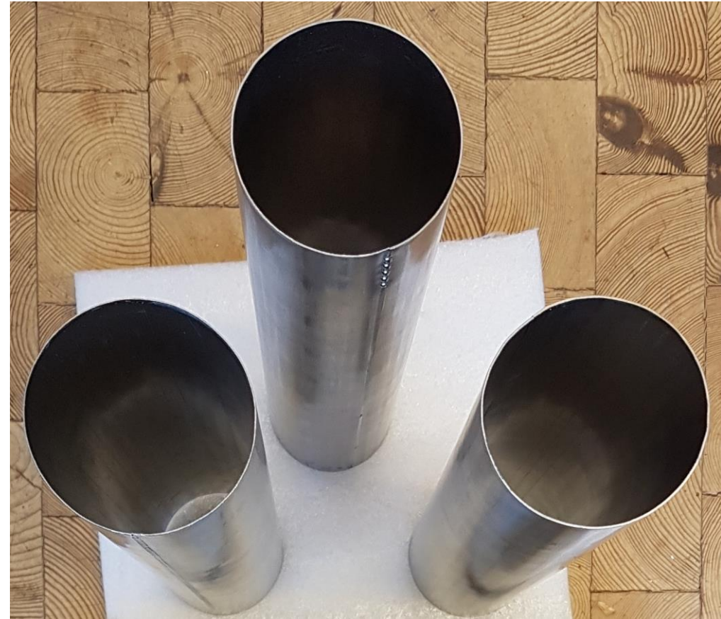
Picture 7: Vacuum pipes welded and rerolled Wall thickness 0,85 mm Inner diameter 77,3 mm
