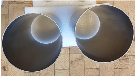
Picture 8: Vacuum pipes welded and rerolled Wall thickness 2 mm Inner diameter 140 mm
