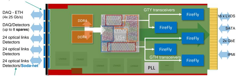
Optical links designed to be operated by LpGBT Soda-net by GTH or GTR transceivers
