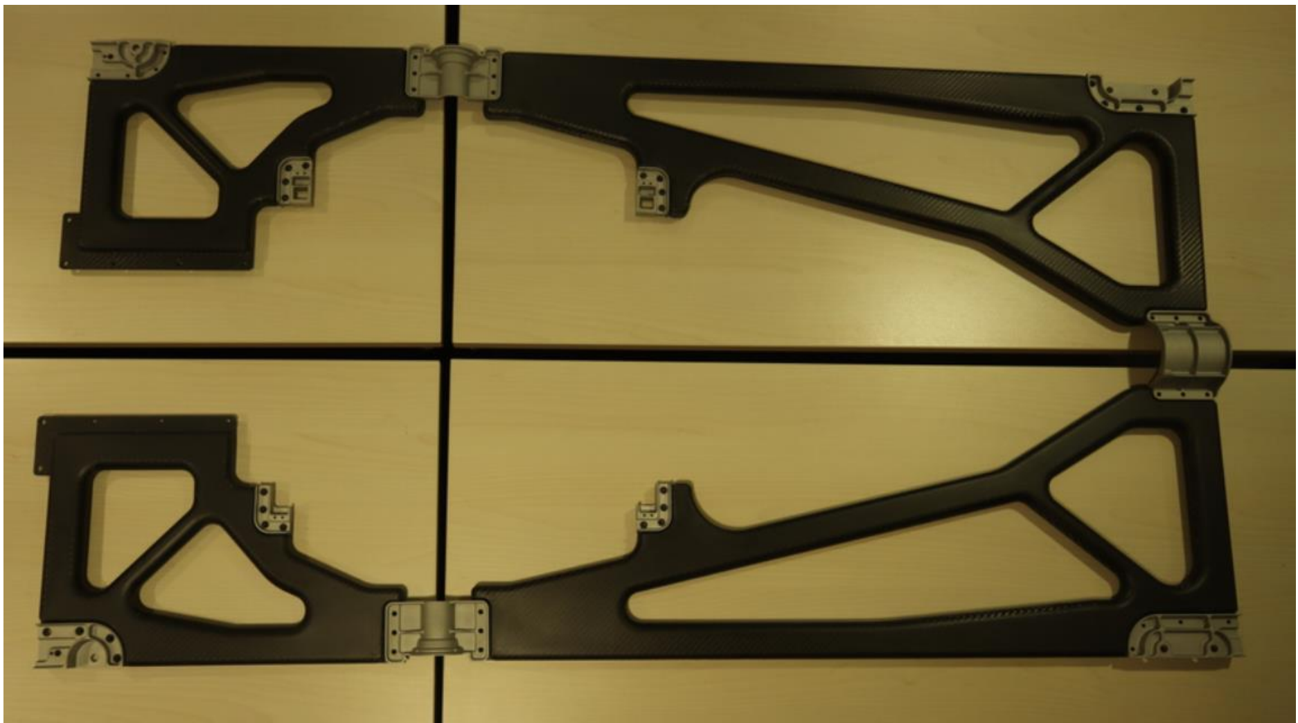
Carbon parts with inner aluminum connectors
