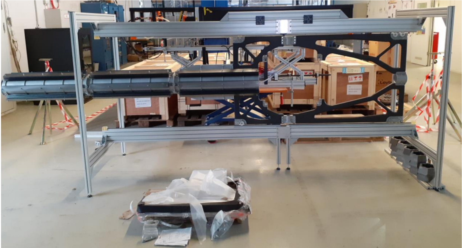
CSF with flat steel bars for load test
