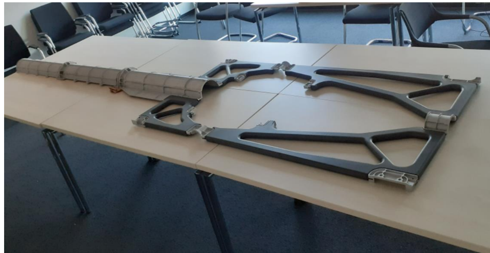
Carbon parts with aluminum connectors and support structure
