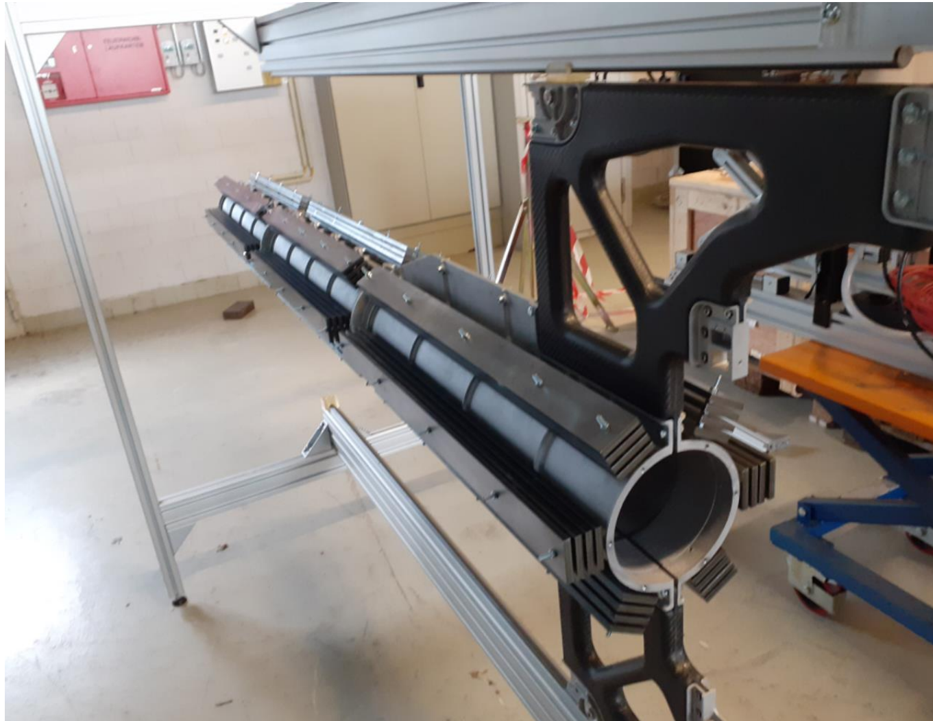
CSF with flat steel bars for load test
