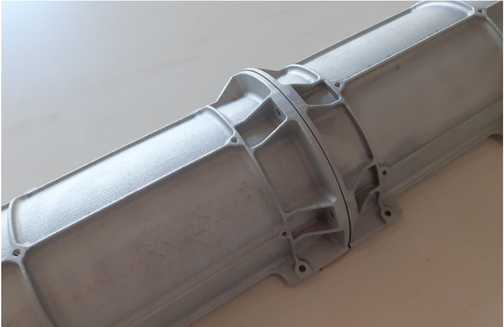
Interfaces between aluminum support structure
