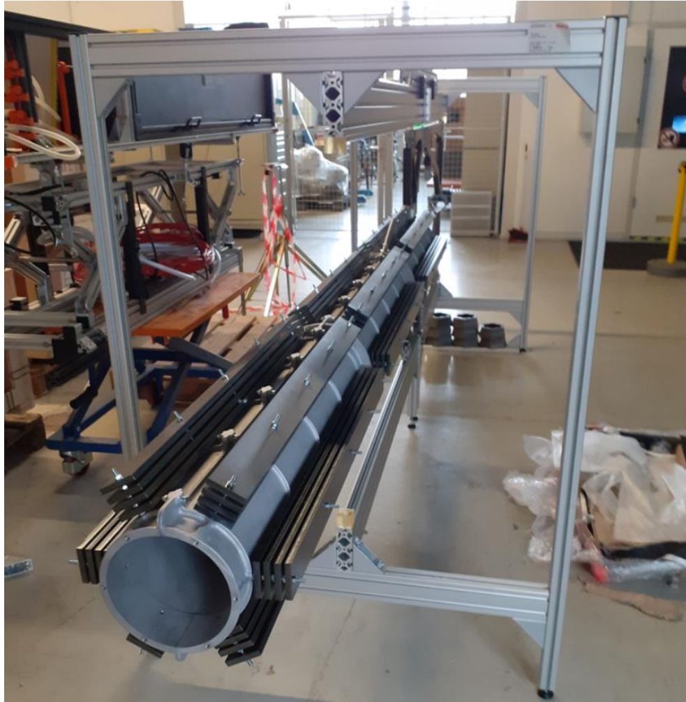
CSF with flat steel bars for load test
