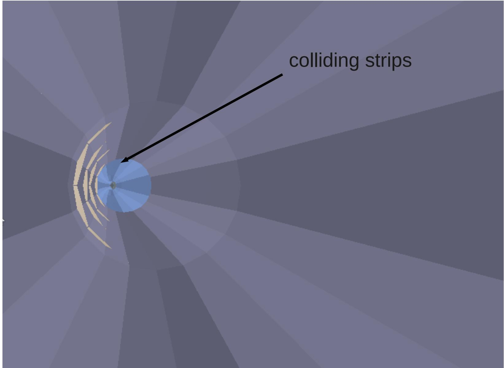
Collision vanishes when dipole beam pipe bending radius is set to 55 m
