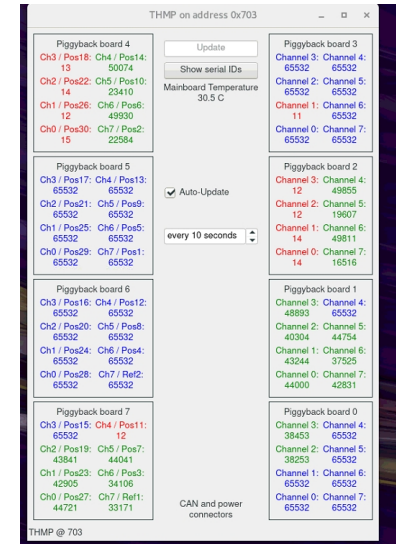
Temp. sensor distribution within alveole
