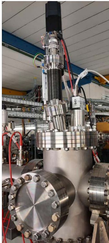
Injector Linac YRT1 Camera & lens with fixed focus and open iris
