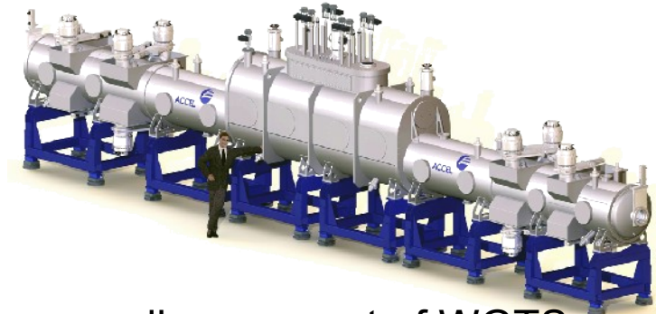
cooling concept of WGTS: pressurized 2-phase Ne
