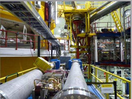
New Hall C Compton : (Diamond Strip e<sup>-</sup> and scintillator photon Detectors) Continuous non-invasive measurement at full current.
