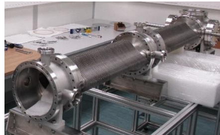
Cryogenic inserts in thin Wall Quadrupole Chamber
