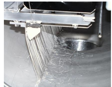
Destroyed SIS18 E-septum wires
