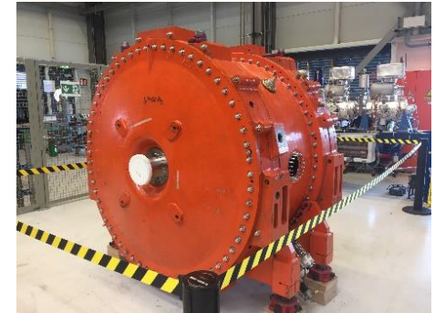
High frequency cavity for micro spill smoothing (proof of principle)
