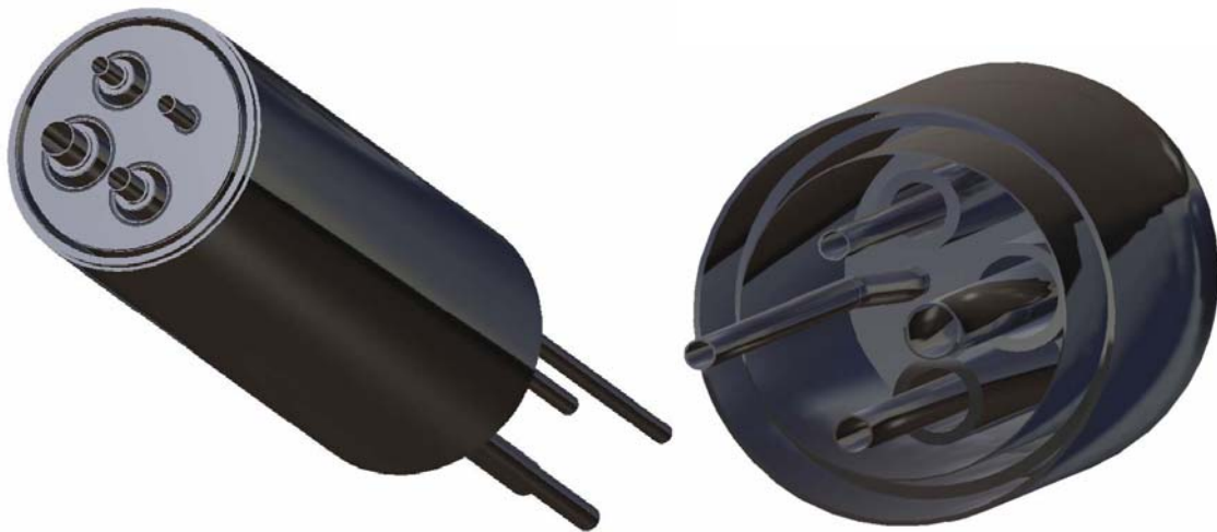
Figure 13. conceptual design of vacuum barrier to separate insulation vacuum among dipole cryostats and feedbox (left: front side; right: rear side)
