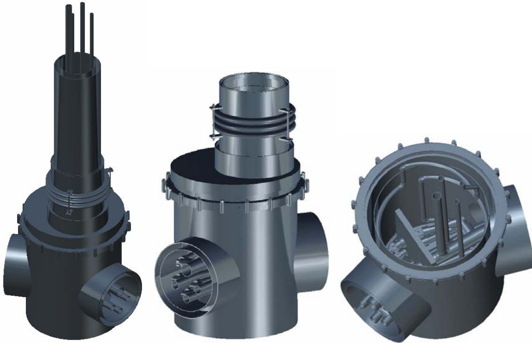
Figure 14. Bend structure for the cryogenic transfer line including the vertical connection line for the feedbox of dipole stage (left: cryogenic transfer line Joint D-1 module and Vertical Connection Line D/M module; middle: cryogenic transfer line Joint D-1 module; right: inner structure of the cryogenic transfer line Joint D-1 module)
