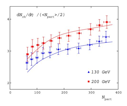
scaled density as a function of  $N_{part}$  at  $\sqrt{s}=130$  and 200 GeV. Data from PHOBOS Collab.
