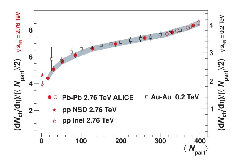
Dependence on the number of participants for Pb-Pb collisions (LHC) and Au-Au collisions (RHIC) - scale difference of a factor 2.1
