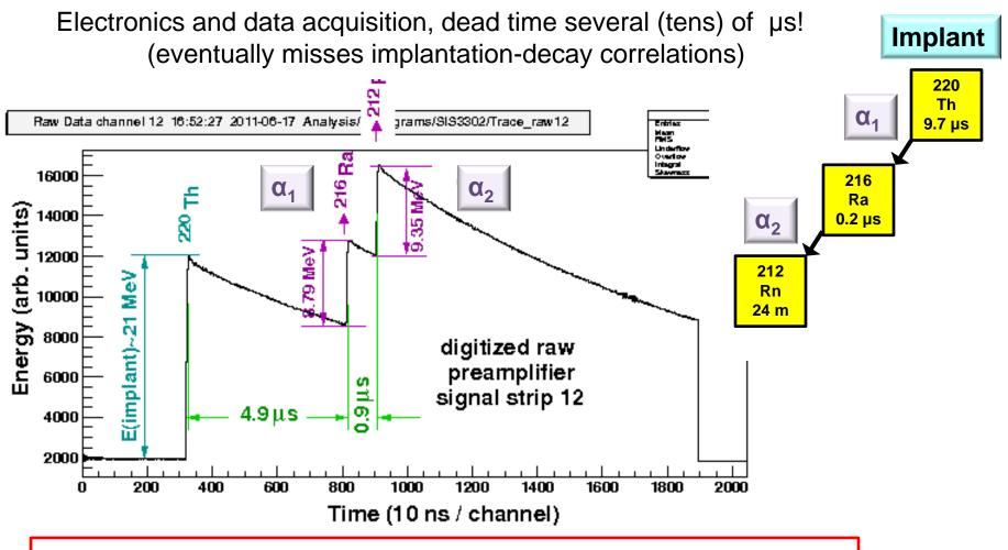
The 2011 *Z*=120 *TASCA* experiment was performed with dead-time free sampling ADC cards developed at GSI-EE N. Kurz *et al*.
