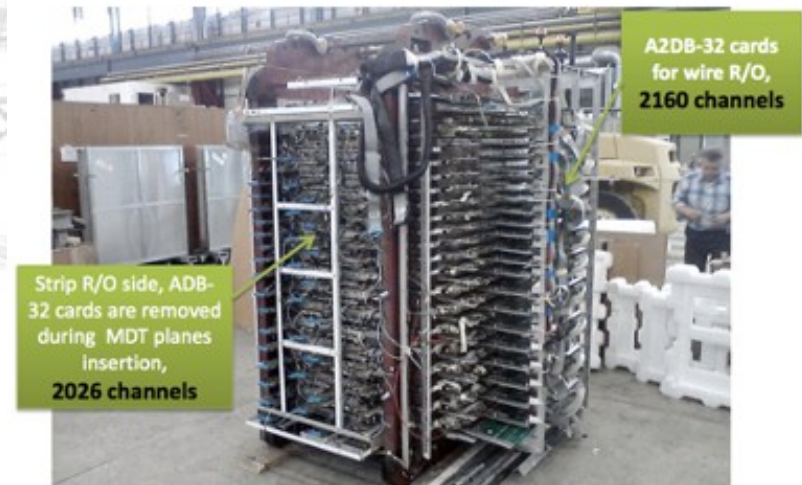
Range System Prototype at CERN mounted for cosmic tests
