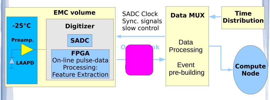
Due to low rates in the barrel EMC and backward EMC extra data-concentration stage has to be introduced
